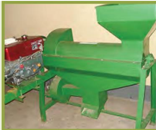
Locally fabricated Non mobile motorised maize sheller
